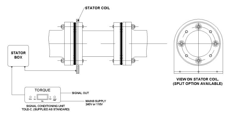
Signal Conditioning Unit (Bench Mounted) Output Options:- 4-12-20mA, +/-10Vdc.
