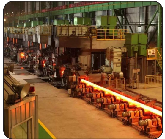
Above: An example of the rolling mill conveyor belts that transport the consecutively produced steel sections through the long manufacturing process. These lines must move at a consistent speed to keep the process moving smoothly.
